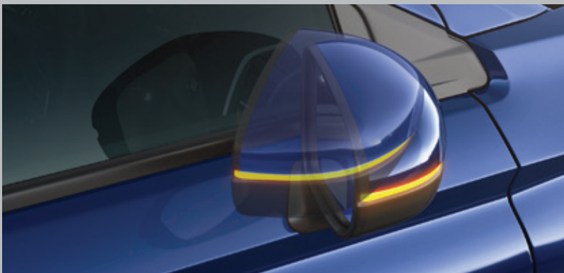
AUTO FOLD DOOR MIRRORS WITH LED TURN SIGNAL
